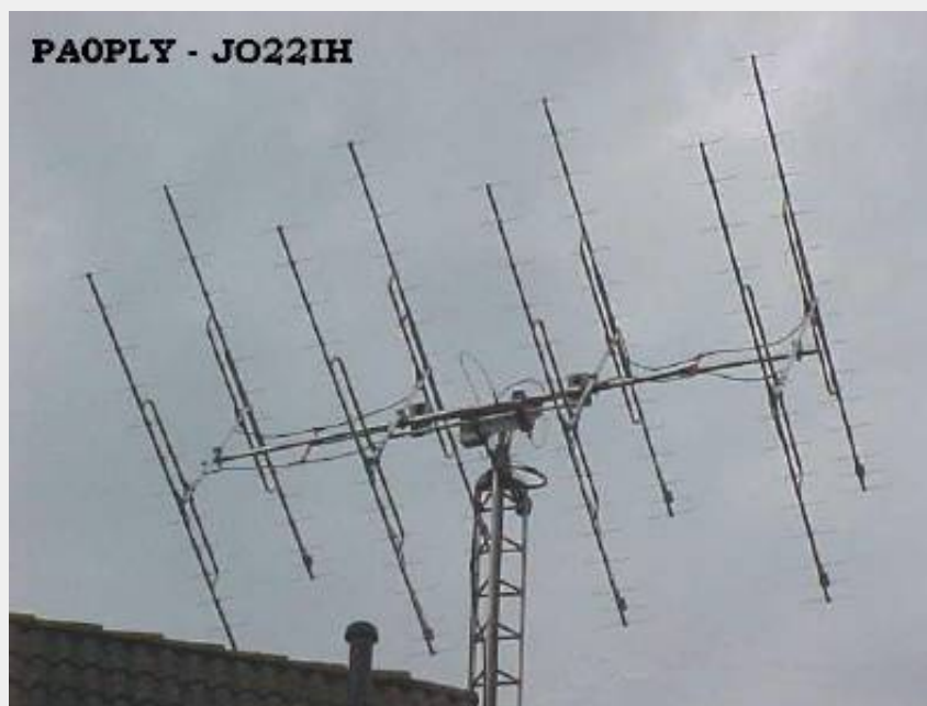
Photo 1.: Large EME array for 432MHz.
