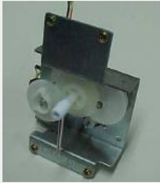
Photo 3: Mechanical indicator needle system
