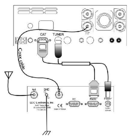
On the FT-847, press the **MENU** button to enter into menu mode. Rotate the **SUB-TUNE** knob until menu #37, "CAT RATE" appears. Rotate the **MEM/VFO CH** knob until "9600" appears. Press the **MENU** button again.
